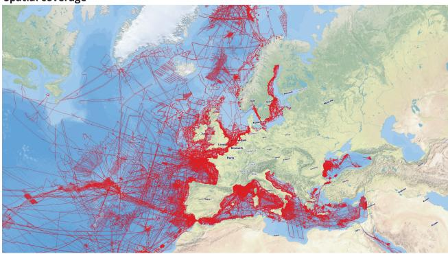
Map indicating the tracks of bathymetric surveys from which datasets have been selected and processed as input for building the overall EMODnet Digital Terrain Model (DTM). The metadata and survey data are gathered from European originators: national hydrographic services, research institutes, and companies. Their coverage goes beyond European waters as scientists collect bathymetry on a global scale.
