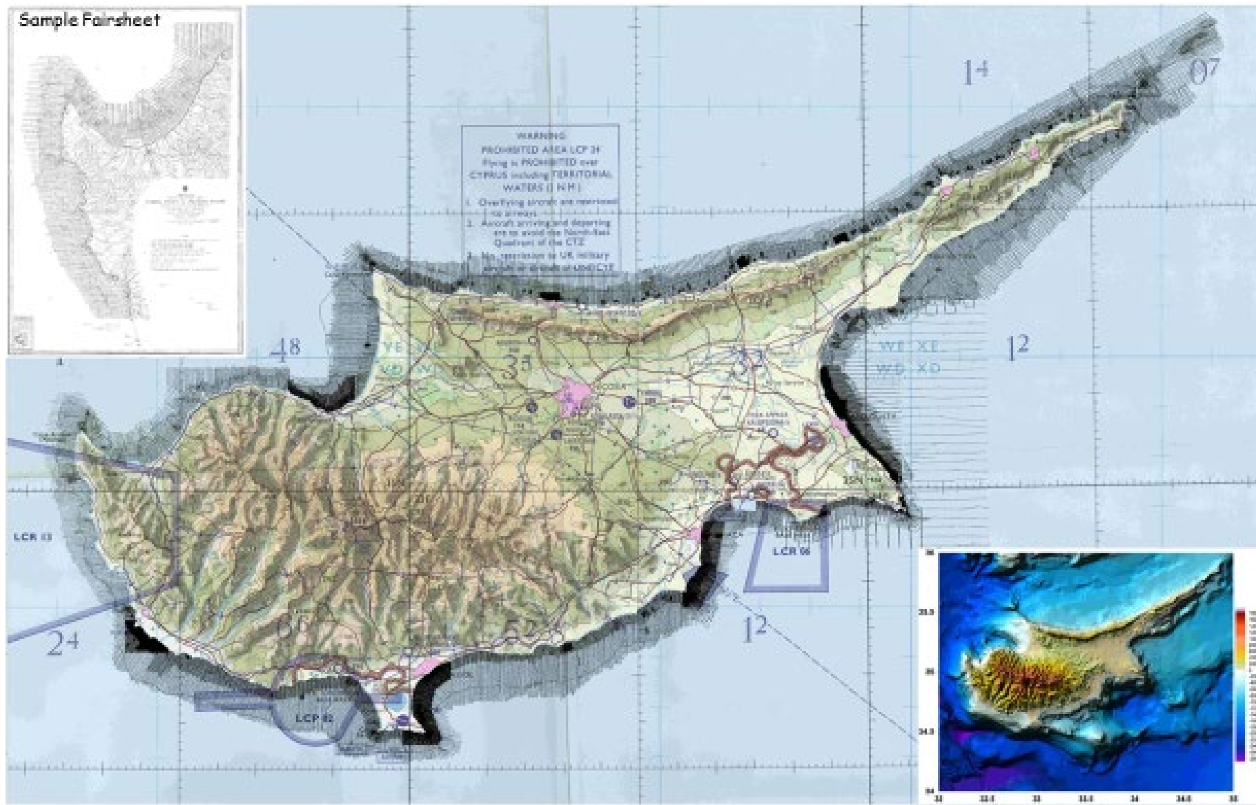
UKHD and UKHO hydrographic surveys around Cyprus in the 1930s and 1950s 183,000 soundings plotted on the 1:500,000 Tactical Piloting Chart
